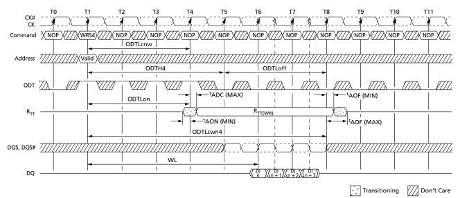
Notes: 1. Via MRS or OTF. AL = 0, CWL = 5.  $R_{TT,nom}$  can be either enabled or disabled. If disabled, ODT can remain HIGH.  $R_{TT(WR)}$  is enabled.
