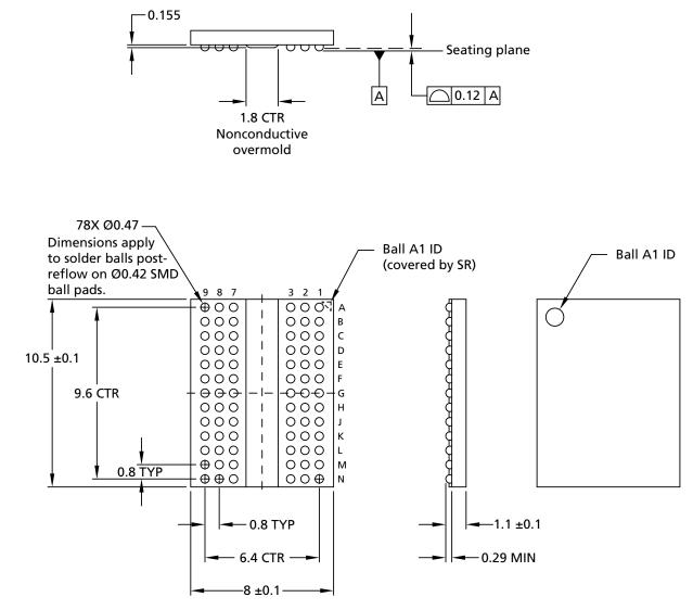
Notes: 1. All dimensions are in millimeters.2. Material composition: Pb-free SAC302 (96.8% Sn, 3% Ag, 0.2% Cu).
