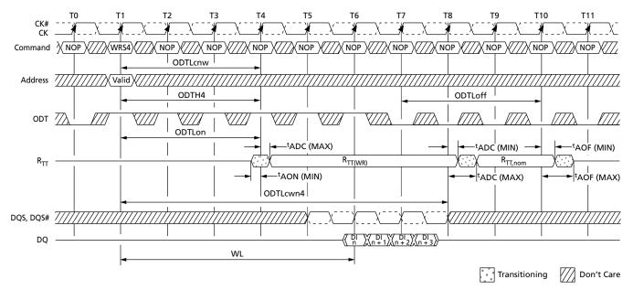
Notes: 1. Via MRS or OTF. AL = 0, CWL = 5.  $R_{TT,nom}$  and  $R_{TT(WR)}$  are enabled.
