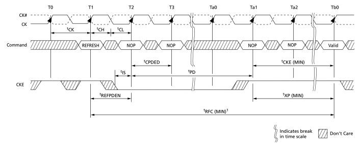
Note: 1. After CKE goes HIGH during <sup>t</sup>RFC, CKE must remain HIGH until <sup>t</sup>RFC is satisfied.
