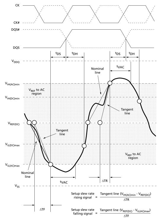
Note: 1. The clock and the strobe are drawn on different time scales.
