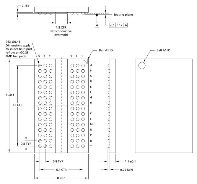
Notes: 1. All dimensions are in millimeters.2. Material composition: Pb-free SAC305 (96.5% Sn, 3% Ag, 0.5% Cu).
