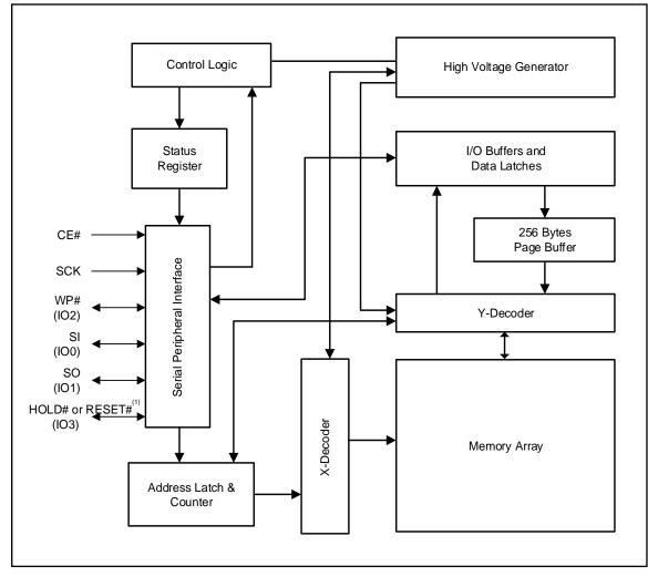
Note1: For RESET# pin option instead of HOLD# pin, call Factory.
